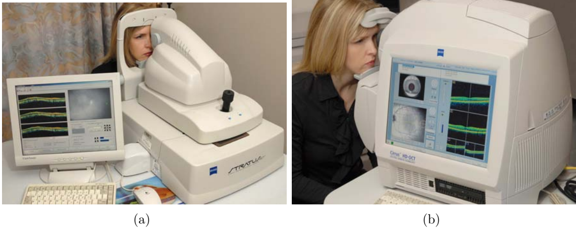
Figure 2.4: Example OCT scanner systems. (a) Stratus OCT-3 (time-domain system by Carl Zeiss Meditec, Inc., Dublin, CA). (b) Cirrus (spectral-domain system by Carl Zeiss Meditec, Inc., Dublin, CA).
